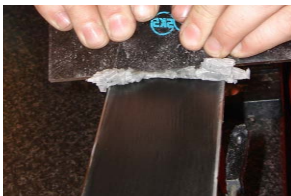
Hot scraping the dirty wax from base
