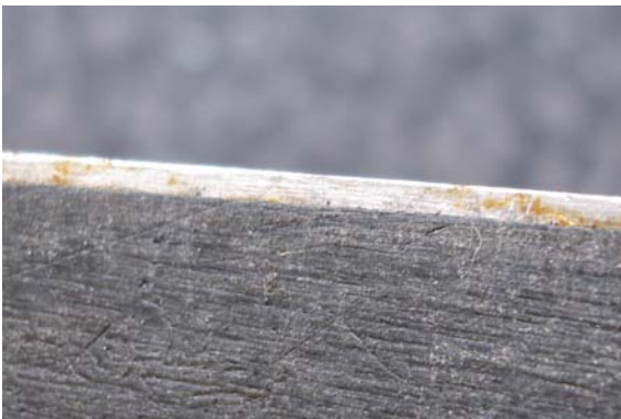
A base edge with nicks and rust
