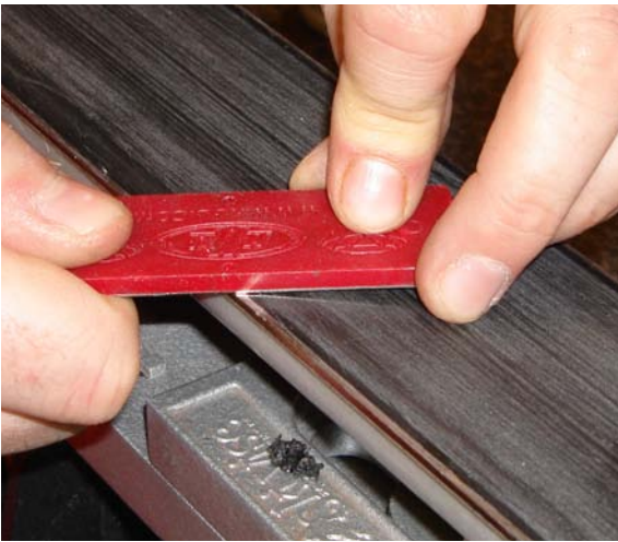
Using a diamond file to remove nicks
