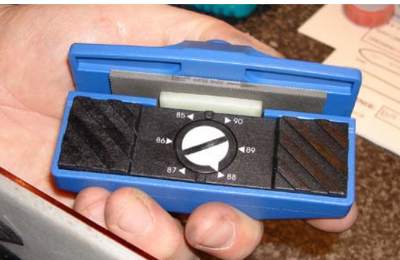
A typical side edge file guide with file
