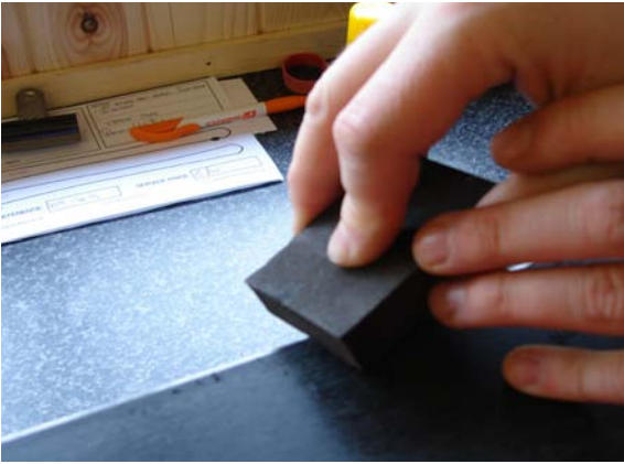
Gummi Stone to remove rust
