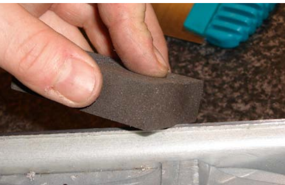
Detuning the edge with a Gummi stone
