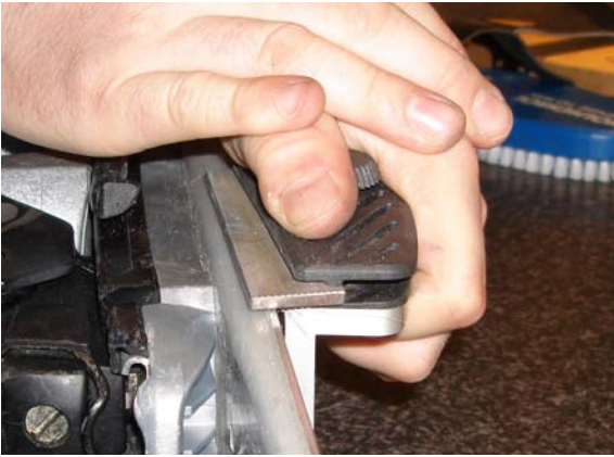
Using the side edge file guide
